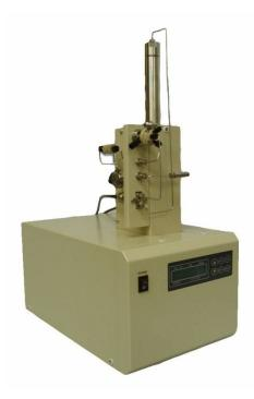
The distinct advantage of the syringe pump is that the pump is able to deliver mobile phase at low flow rate with very low pulsation. The model 8522 Syringe Pump can be used for delivering solvent for which precise flow rate and low pulsation are required and delivering high viscosity solvents.
