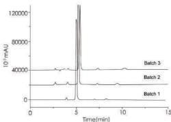
From the results above, multiple batches of column were selected to test the column, showing Blossmate SAX column has excellenet reproducibility and stability.
