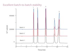
From the results above, multiple batches of column were selected to test the column, showing Blossmate PSV C18 column has excellent reproducibility and stability.
