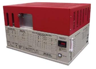
Up to six detectors can be installed on the same 8610C GC.
