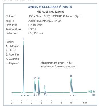
In spite of the polar character of the embedded functional group NUCLEODUR® PolarTec exhibits sufficient hydrophobic properties and is very well suited for analyzing basic compounds.
