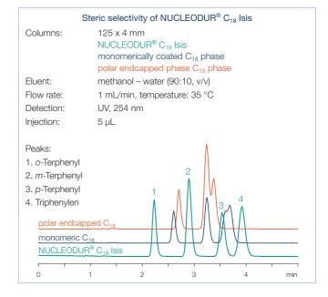
The separation of o-terphenyl and triphenylene is a good example to evaluate the selectivity of a RP column in terms of the shape of two molecules. The phenyl rings of o-terphenyl are twisted out of plane while triphenylene has a planar geometry. The separation factor  $\alpha$  is a measure for the steric selectivity. As is shown below the  $\alpha$  value is considerable larger on NUCLEODUR  $^{\!8}$  C  $_{\!18}$  lsis compared to a conventional C  $_{\!18}$  column.
