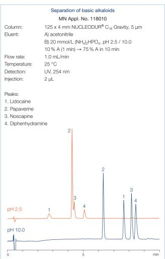
The following chromatogram demonstrates the stability of  $\mbox{NUCLEODUR}^{\mbox{\tiny 8}}$   $\mbox{C}_{\mbox{\tiny 18}}$  Gravity under alkaline conditions. The ultrapure Gravity with its unique high density surface bonding technology withstands strong alkaline mobile phase conditions.
