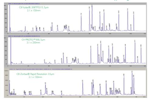
Superior Resolution with PROTO™300 C4 for Protein Tryptic Digests
